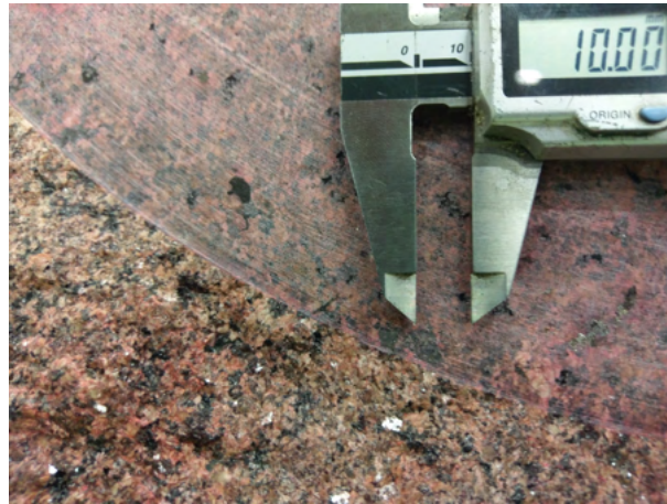
Figure 41: The granite used for the experiment; shown are a sawed and a broken section, although this piece is just a demonstration to show the grain size better, and the actual test blocks had no smooth sawed of section prior to testing.
