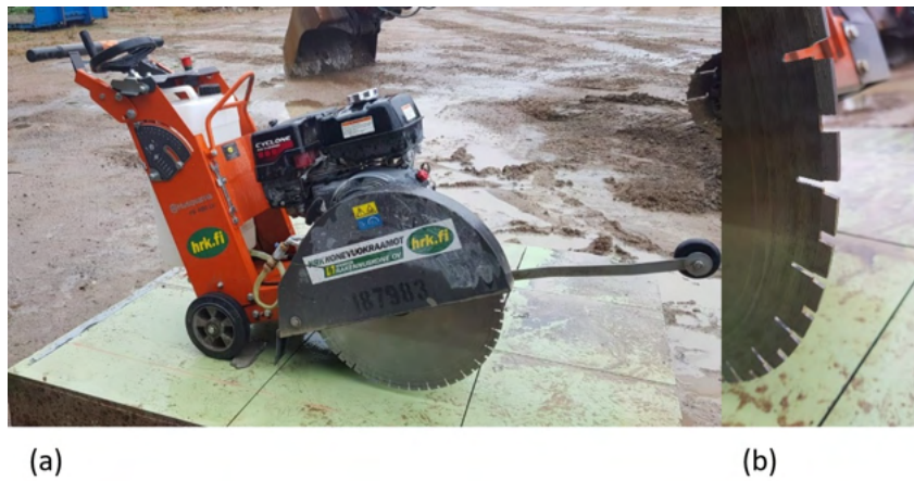
Figure 43: Pictures showing (a) the diamond saw used and (b) a close-up of its diamond-tipped blade.
